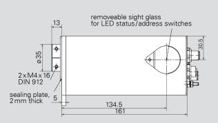
hollow shaft ø14H7/20 depth with clamp and feather key DIN 6885-A5x5x12
