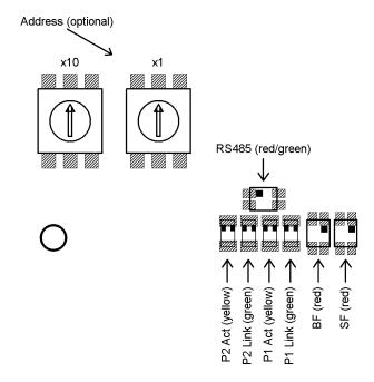
The LEDs are visible through two windows even when the bus adapter cover is closed.
