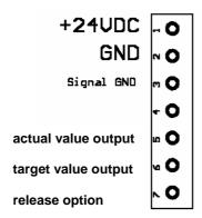
Pins 1 (+24VDC) and 2 (GND) are for connecting the required operating voltage; pin 3 (signal GND) is for the ground for the target and actual values. Pin 4 (actual value output) is for a signal of 0 ... 10 V (or 4 ... 20 mA, depending on the design) and can, for instance, be used to connect an instrument for taking measurements. Pin 6 (target value input) is for a signal of 0 ... 10 V (or 4 ... 20 mA, depending on the design) and is used for positioning the gear.
