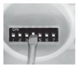
Any dosage required can be set via DIP switch combinations
