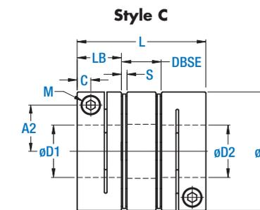
The shafts of the equipment (up to the maximum bore size of the coupling) may be extended into the interior of the coupling without any modification to the ServoClass coupling. However, the ends of the shafts must never touch each other.
