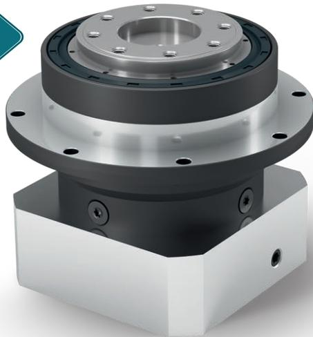
The **PFHE** represents an economically attractive alternative for high-load applications in which high radial loads occur. The combination of special pre-stressed inclined roller bearings and a flanged output shaft in accordance with EN ISO 9409-1 gives the **PFHE** a very high load capacity. Thanks to the radial shaft seal that is used, this gearbox achieves protection class IP65 at the output side and can therefore also withstand adverse usage conditions.
