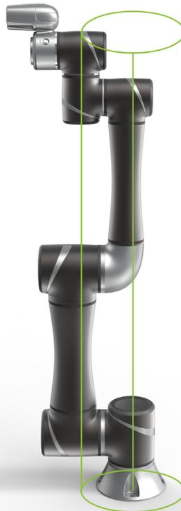
Joint coordinate system and  $d_{\text{offset}}$  definition.
