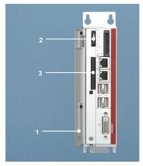
Opening the front flap (1) allows access to the battery (2) and the Flash storage medium (3). Optionally the Industrial PC can be fitted with a second Flash medium or only with one hard disk.
