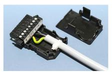
Fix the upper part of the strain relief housing by snapping it onto the lower part.
