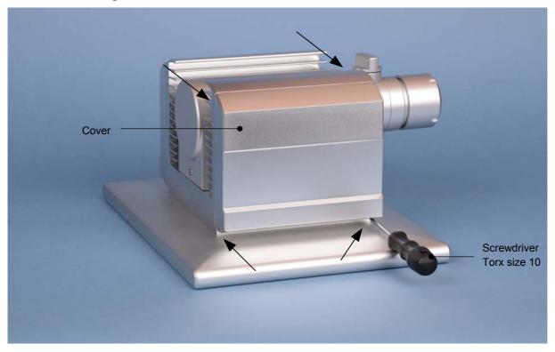
After unscrewing the four screws (see arrows) with a star screwdriver Torx size 10 the drive cover can be taken off.
