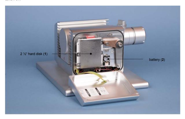
Removing the cover allows access to the hard-disk (1) and the lithium battery of the system clock (2). The hard-disk drive can now be pulled out. Here, changing the lithium battery is also possible.
