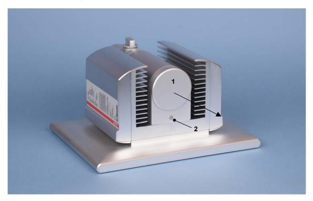
First loosen the fixing screw (2) with a star screwdriver Torx size 20. The cover now can be drawn off in direction of the arrow (see next picture).
