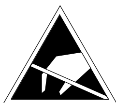
Figure B-1 Symbol for identification of electrostatic sensitive devices
