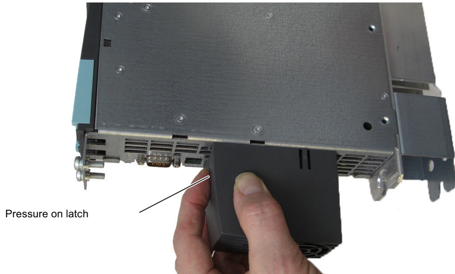
Figure 7-3 Unlatch the double fan/battery module
