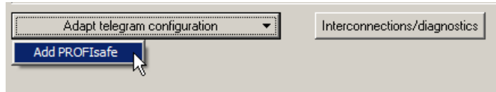
Figure 6-33 Adding the PROFIsafe telegram on the drive
