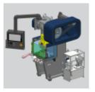
This application example allows you to simulate the SIMATIC Simapress application in combination with the SIMATIC S7-F/P Press Safety Blocks using PLCSIM Advanced, SIMIT and NX Mechatronics Concept Designer (MCD).
